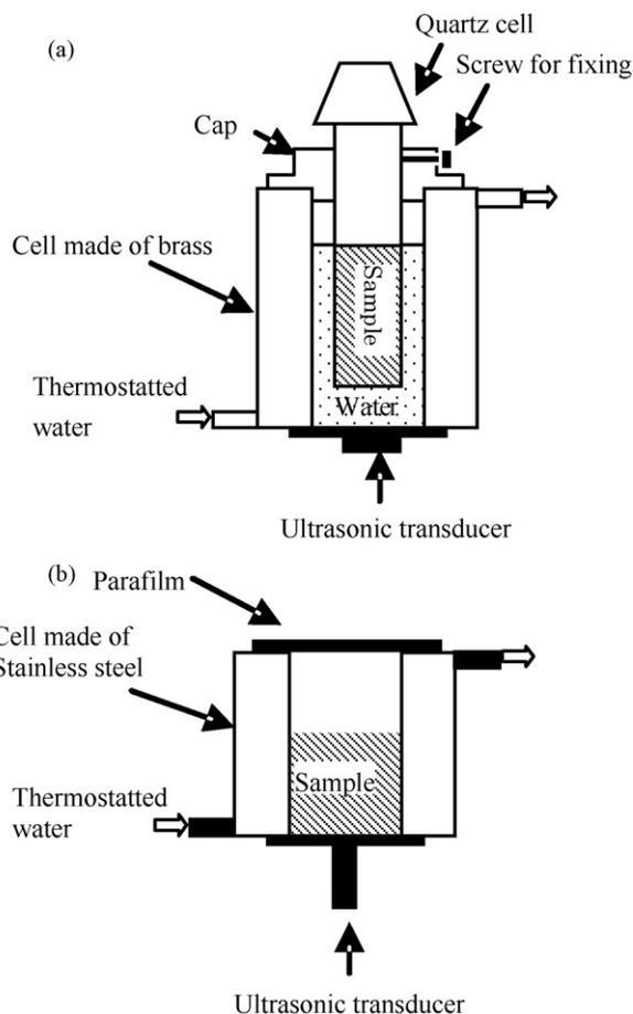
Fig. 1. The illustrations of the ultrasonic baths used for (a) high-frequency (480 kHz) and (b) low-frequency (43 and 133 kHz) experiments.
